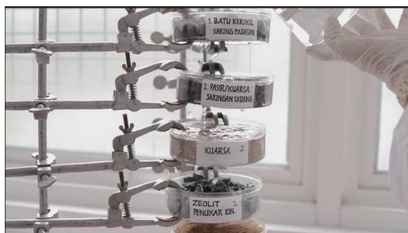
Figure 2. Processing of liquid waste from the biology laboratory at school A
