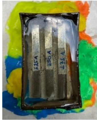
Gambar 5. Proses mounting uji kekerasan
