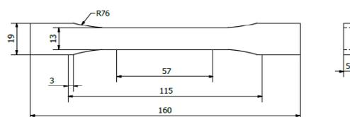
Gambar 2. Spesimen Uji Tarik ASTM D638
